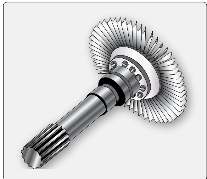
Figure 1-64. Rotor elements of the turbine assembly.
