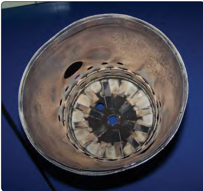
Figure 1-53. Inside view of a combustion chamber liner.
