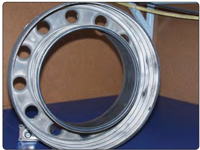
Figure 1-58. Annular combustion chamber with ceramic coating.
