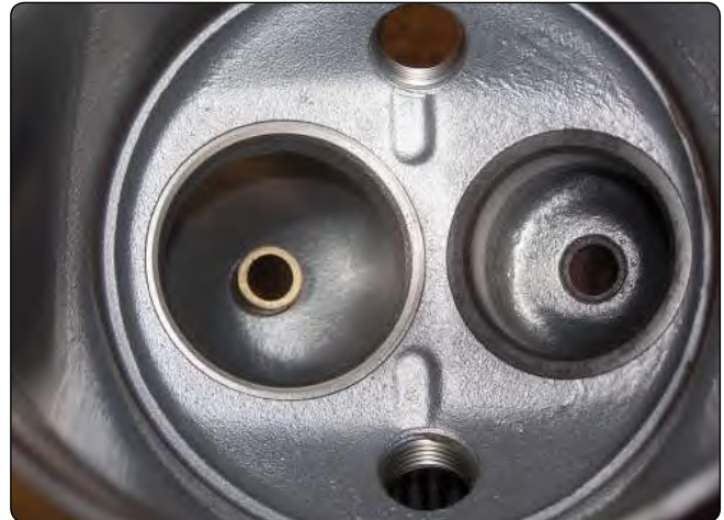
Figure 1-21. View of valve guide installed on a cylinder head.
